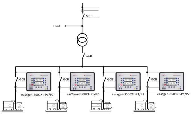
4 x 1000 kVA Caterpillar Diesel generator sets paralleled within 7 seconds
