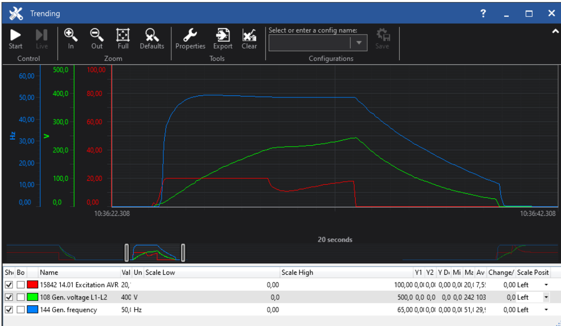
Figure 2.2: This is a trending example which shows that on one side the excitation current is strong enough to build up a generator voltage, but the generator voltage needs too long time to come into the generator operating range window. The generator undervoltage monitor stops the engine.
