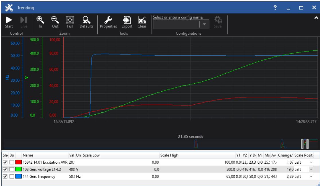
Figure 2.3: This is a trending example which shows that with fast ramping (“ID5633 Starting ramp” = 100%. ) the generator voltage reaches the setpoint but also after too long time. It does not come to a shut down of the engine because the generator undervoltage monitor was delayed on 30 seconds.
