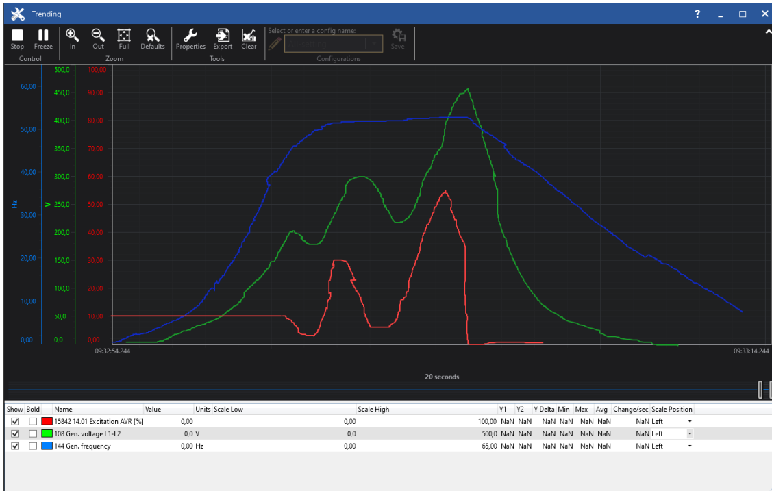
Figure 3.2 (Sketch): This is a trending example which shows that the generator voltage is clear influenced through the AVR but after some generator voltage swings it comes to a generator overvoltage. The engine is stopped.
