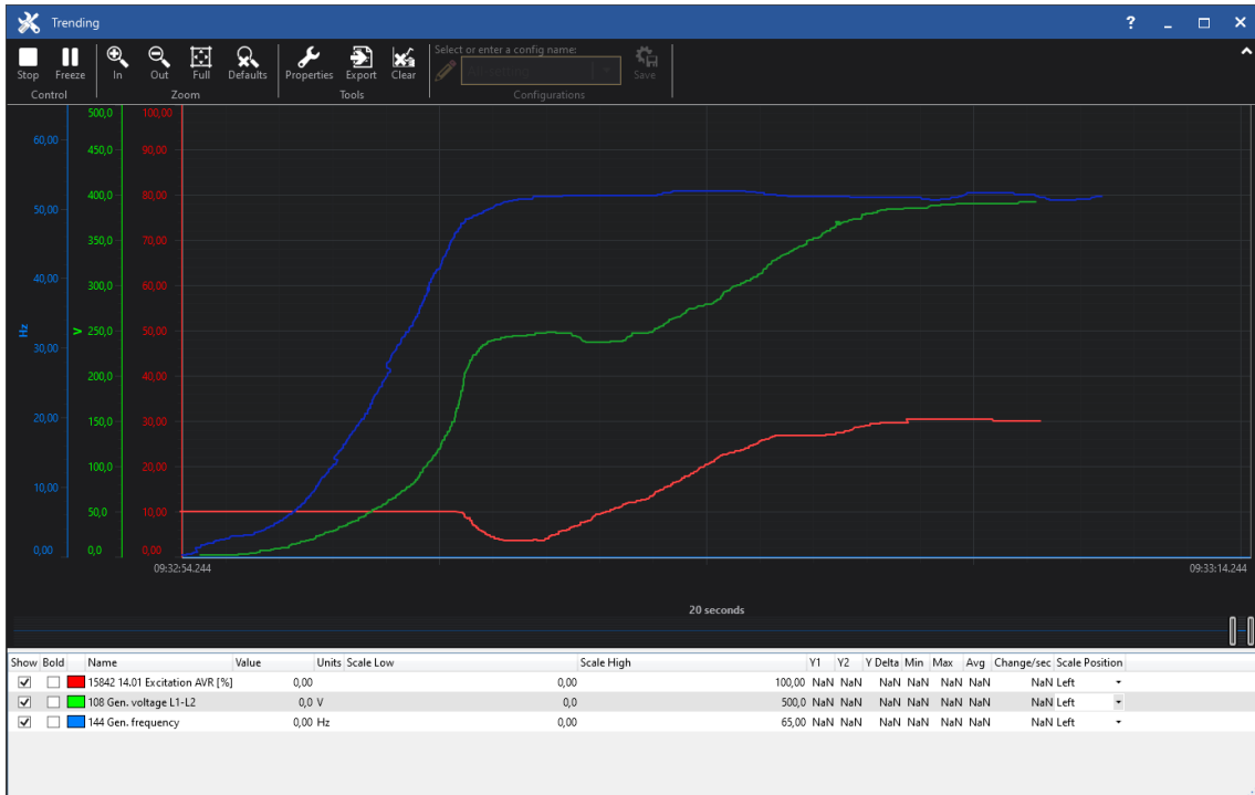
Figure 3.4 (Sketch): This is a trending example which shows that the generator voltage is stocked during startup phase.
