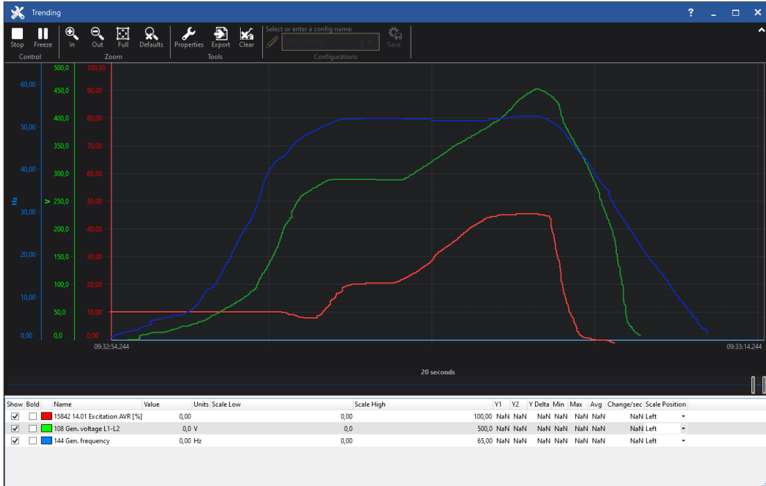
Figure 3.3 (Sketch): This is a trending example which shows that the generator voltage is buildup not so bad but ends as well in an overvoltage situation. The engine is stopped.
